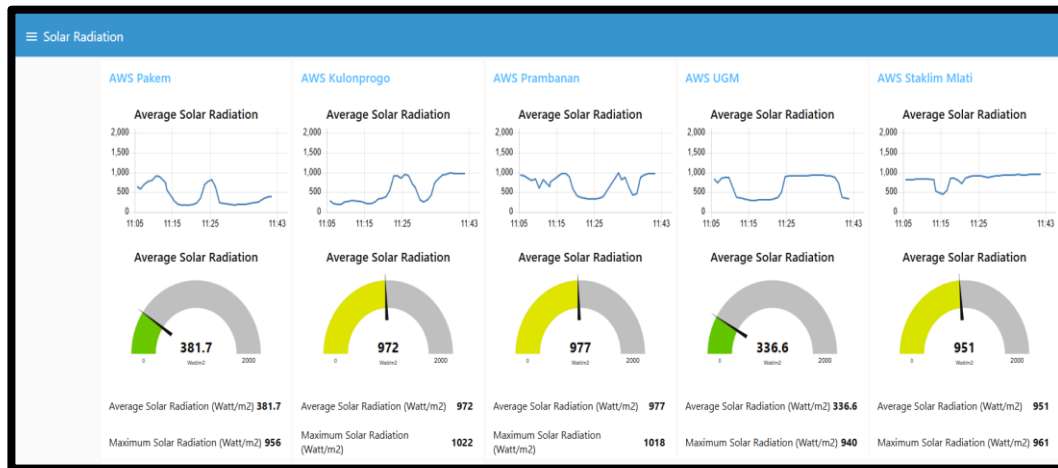
Figure 10. Display Data of Solar Radiation of AWS network in Yogyakarta
