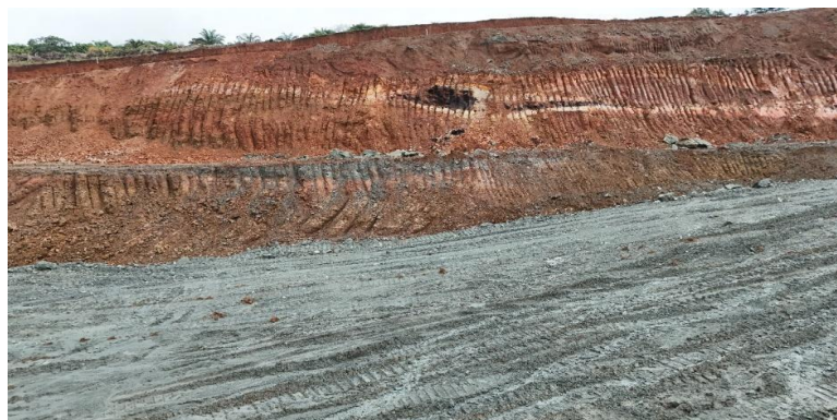
Figure 3.1. Normal bench with no potential slope failure.
